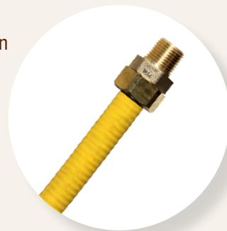
Flexible natural gas connectors are corrugated metal tubes that attach gas appliances to a home or building's natural gas supply pipes. Some older, uncoated brass flexible gas connectors are still in use and can corrode or break. Be cautious when moving an appliance to check the gas connector. This may cause the connector to break, potentially resulting in a gas leak or fire.
